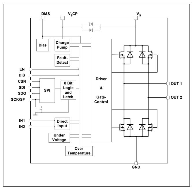
Figure 2 Block Diagram TLE 7209-2R
