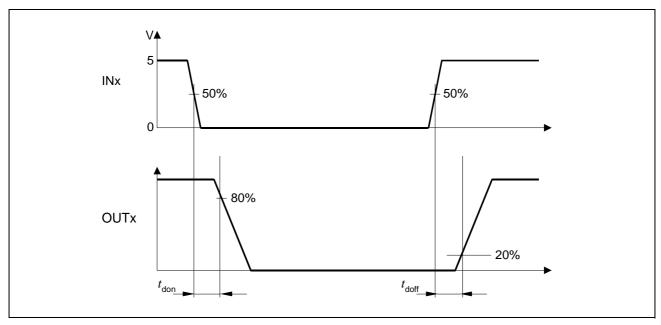
Figure 10 Output Delay Time
