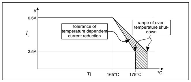
Figure 4 Temperature dependent current reduction
