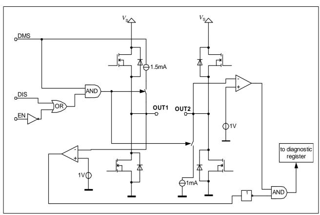
Figure 9 Functional block diagram of open-load detection
