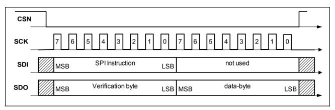
Figure 8 SPI communication
