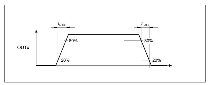
Figure 12 Output Switching Time
