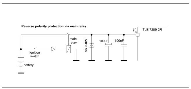
Figure 16 Application Examples for Over-Voltage- and Reverse-Voltage Protection
