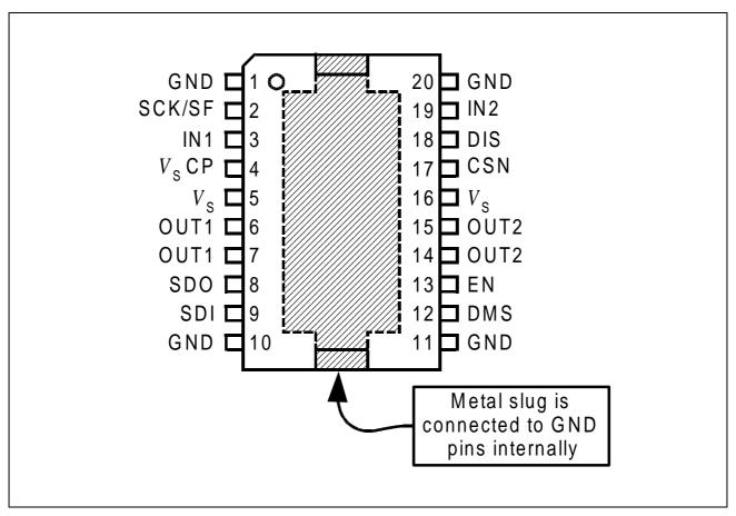
Figure 1 Pinout TLE 7209-2R
