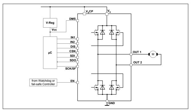
Figure 14 Application Example with SPI-Interface
