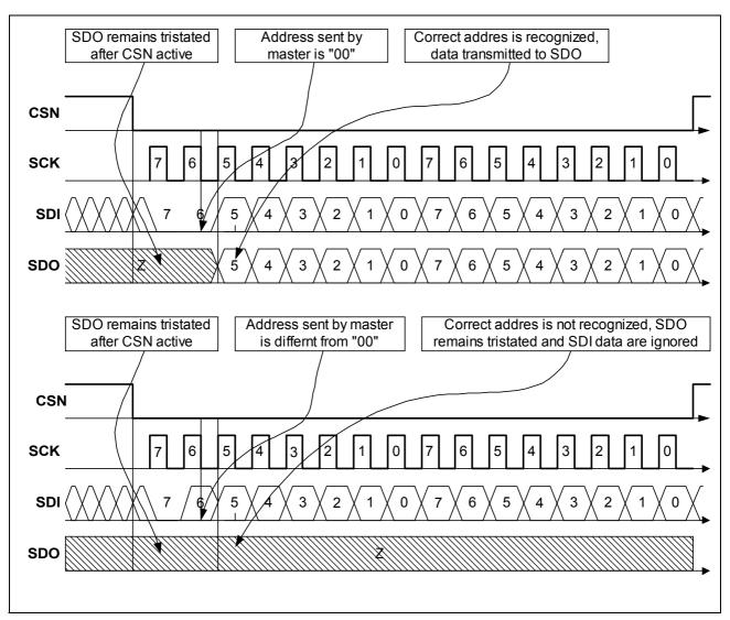
Figure 7 Bus-arbitration by chip-address
