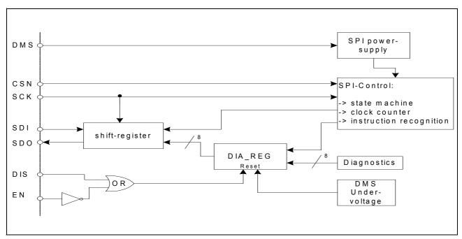
Figure 6 SPI block-diagram
